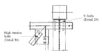
Beam-Column Connection for Truss Structure Example 18
